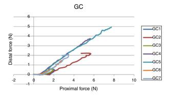
**Figure 4** Results of pushability and force transmission measurements of the catheters. DC: diagnostic catheters; GC: guide catheters.
