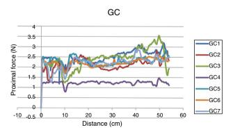
**Figure 5** Results of trackability measurement of the catheters by force-distance curves. DC: diagnostic catheters; GC: guide catheters.
