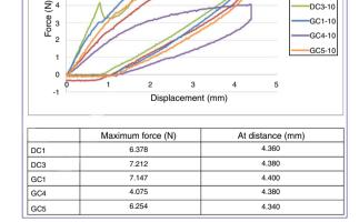
**Figure 7** Results of three-point bending test measured at 4.5 and 10 cm from the distal tip with maximum force distance parameters. DC: diagnostic catheter; GC: guide catheter.
