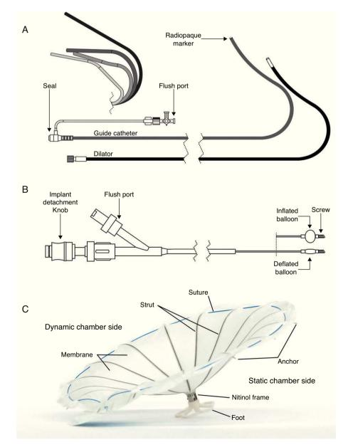
Figure 1 Components of the Parachute device (detailed description in text). (A) Guide catheter and dilator; (B) access system; (C) the Parachute implant.
